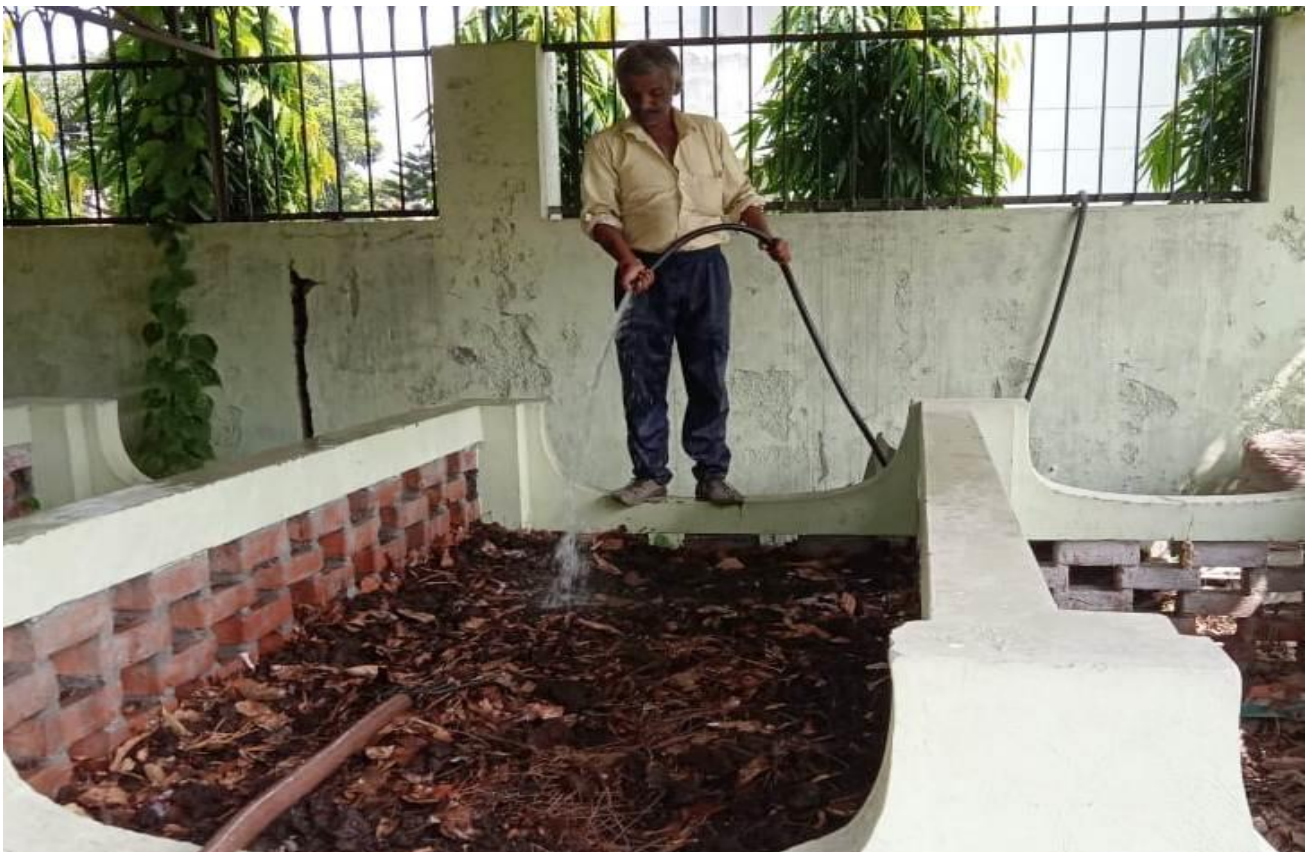
Garbage mixed and watered in the composting pits for proper maturity
