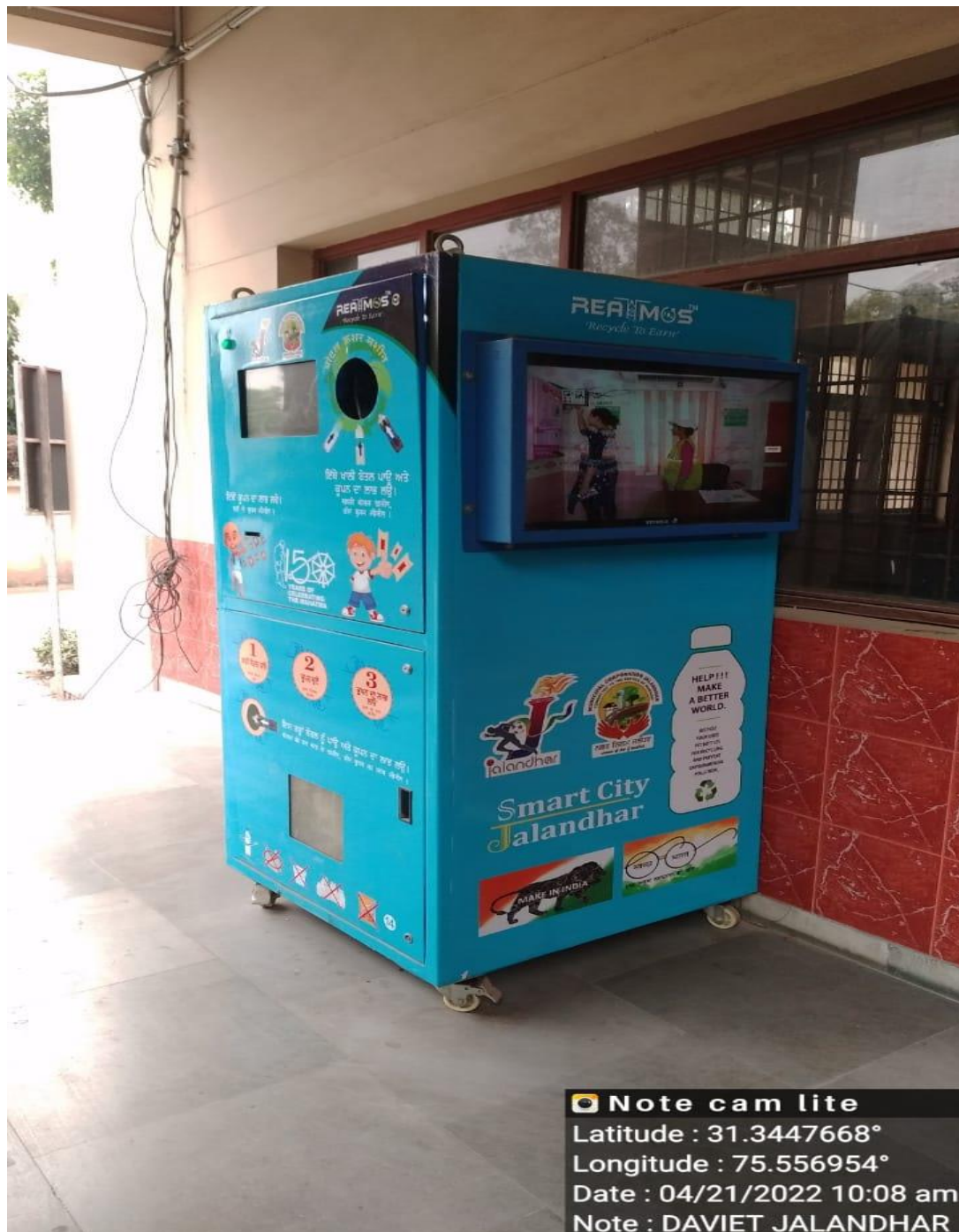
Plastic Bottles Crushing and waste recycling machine installed in DAVIET, Jalandhar
